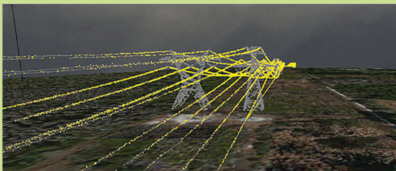
Points representing powerlines can be automatically reclassified
