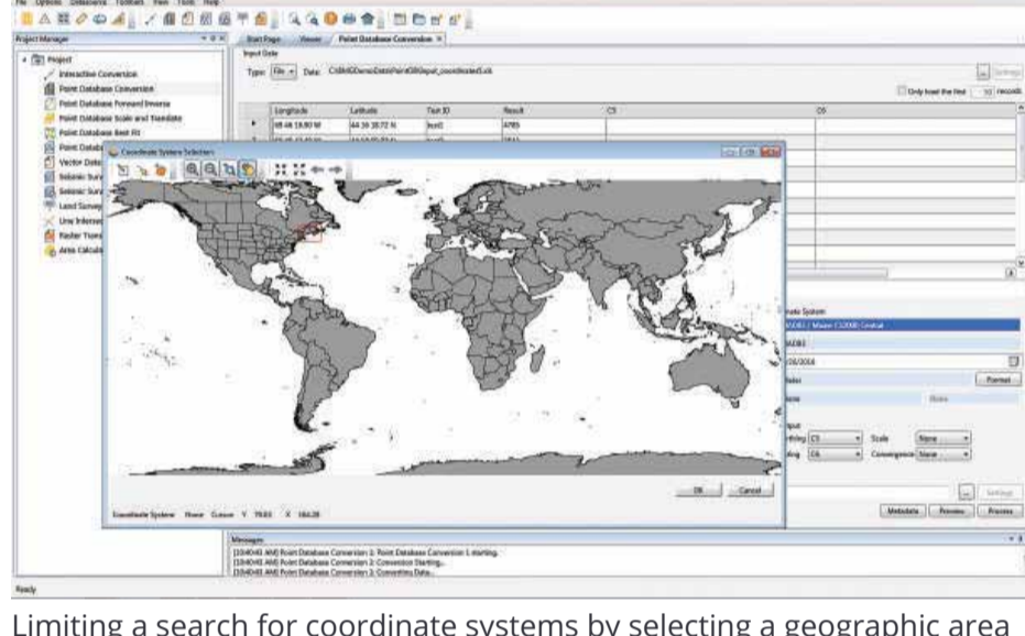
Limiting a search for coordinate systems by selecting a geographic area before processing a point database conversion job
