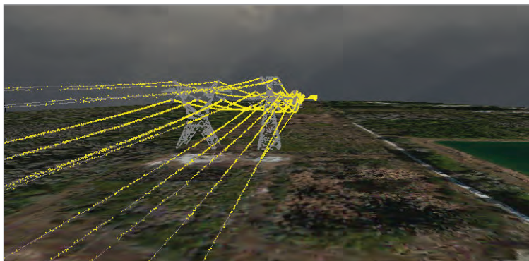
LiDAR points representing powerlines can be automatically reclassified.
